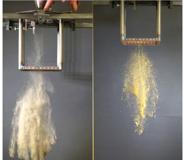
Comparison of untreated soil(right) and treated soil(left) falling through air.
