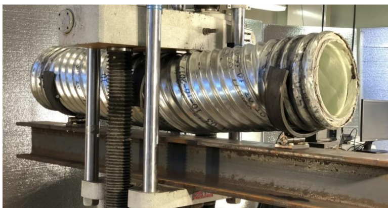
Full-scale laboratory testing of GFRP-lined metal culvert
