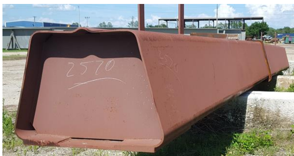
SPGS test specimen prior to deck prefabrication
