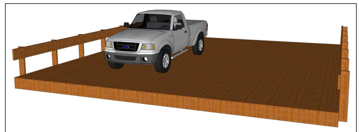
Figure 2. Glulam slab timber bridge. (by: Zach Carnahan)
