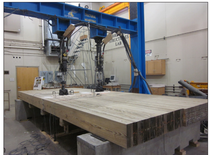
Figure 4. Glulam slab bridge test specimen. (Photo credit: Zach Carnahan)
