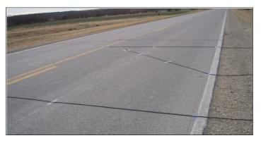
Set up of Road Tubes Sensors for Data Collection on Vehicles' Lateral Position
