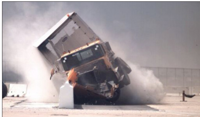
Figure 3. A crash test of the new concrete median barrier. Note that the design is more vertical than standard designs, which reduces the probability of the vehicle "climbing" the barrier and rolling over.
