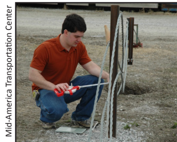
Figure 2. Cody Stolle, a MATC graduate student at the time of this picture, measuring a cable median barrier prior to a crash test. Now a Post-Doctoral Research Associate at the Nebraska Transportation Center’s Midwest Roadside Safety Facility, Stolle was honored as MATC Student of the Year for his contributions to this research project.
