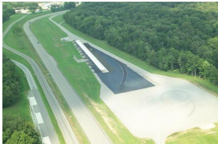
Figure 1.4-2: Navistar Proving Grounds Vehicle Dynamics Pad with High Speed entrance from Oval Track, Low Coefficient Surfaces and 500' Radius
