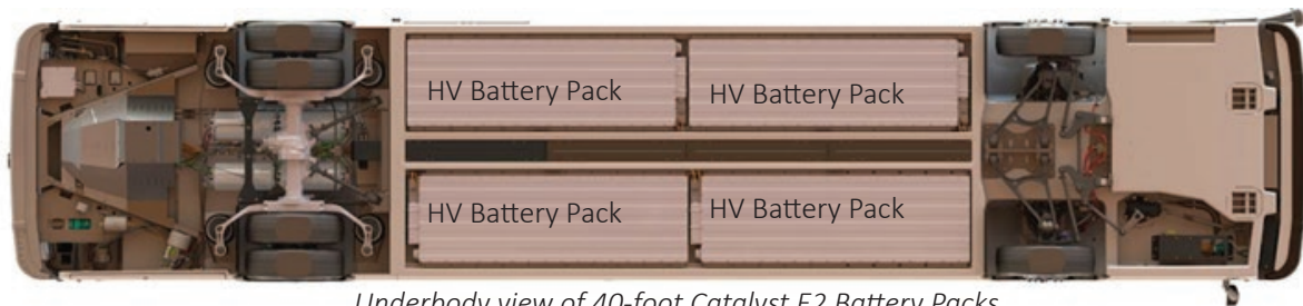
Underbody view of 40-foot Catalyst E2 Battery Packs
