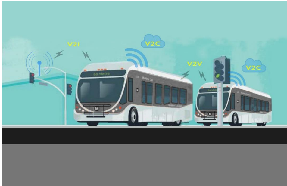
Figure 2. V2X Communications for BRT Operations
