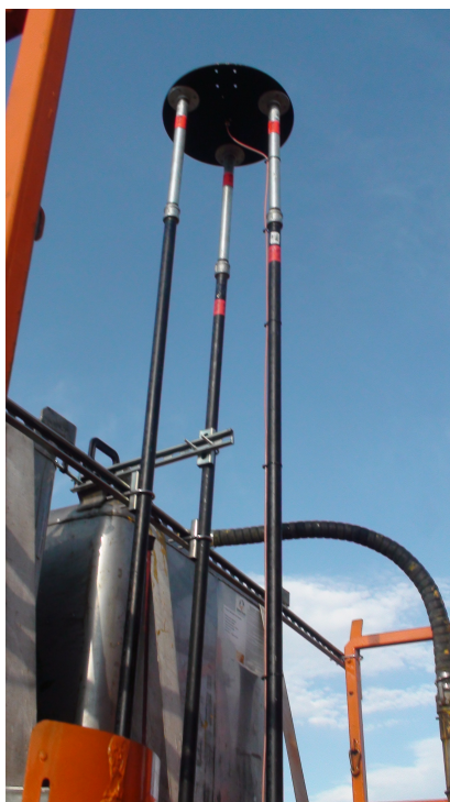
Figure 19: RTK Antenna located on the follower vehicle
