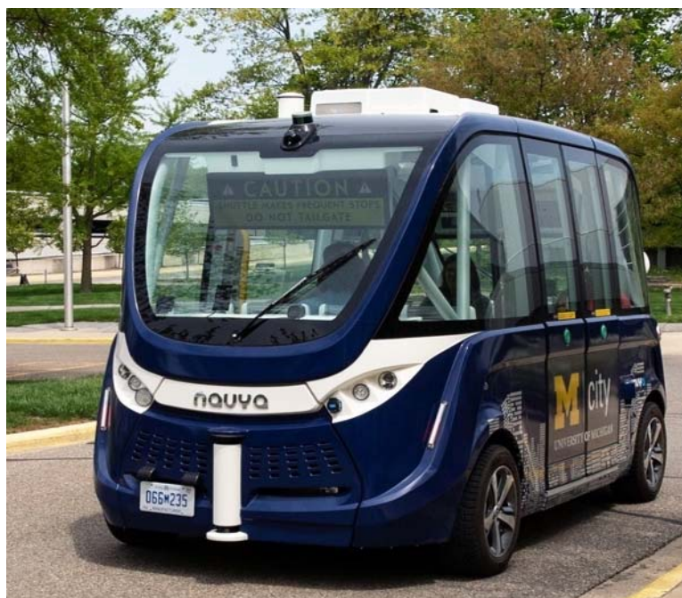
Figure 9: The caution screen is an example of an e-HMI used by EasyMile, an autonomous shuttle company. This screen alerts nearby road users and pedestrians of the vehicle's intent and state. In this example, the vehicle is communicating it makes frequent stops and advises surrounding road users to not follow too closely.
