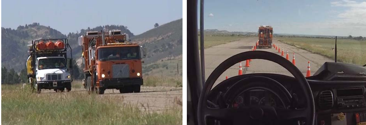
Figure 21: Field tests conducted by CDOT in 2017 on a defunct airfield (closed course track) owned and operated by Colorado State University. (Left: external view of the leader/follower during the field tests. Right: View of the inside of the automated truck mounted attenuator vehicle).
