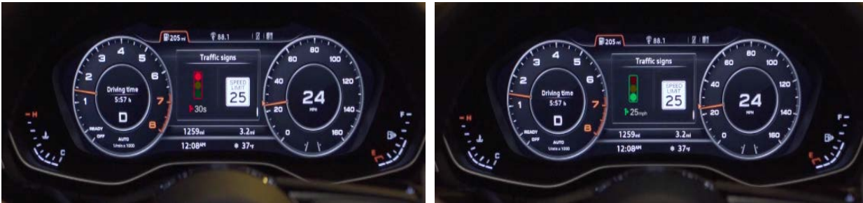
Figure 14: Traffic signal information, on the market since 2016, now also includes GLOSA
