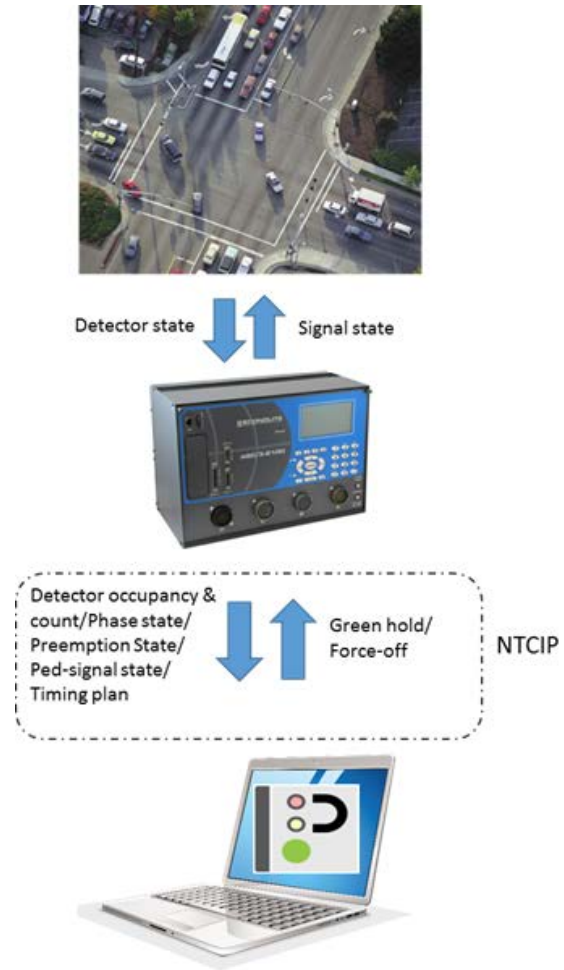
Figure 15: Communication to traffic signal controller for second-by-second control decision update
