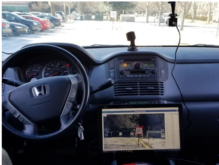
Figure 7: Prototype machine vision system for CAVs with a dash cam attached to the vehicle windshield for real-time barcode signage reading.
