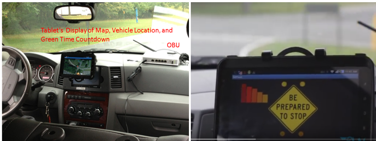
Figure 4: Lear OBU unit instrumented inside a passenger car for testing red light violation warning application (a) setup inside the vehicle, (b) example warning message displayed with sound alert
