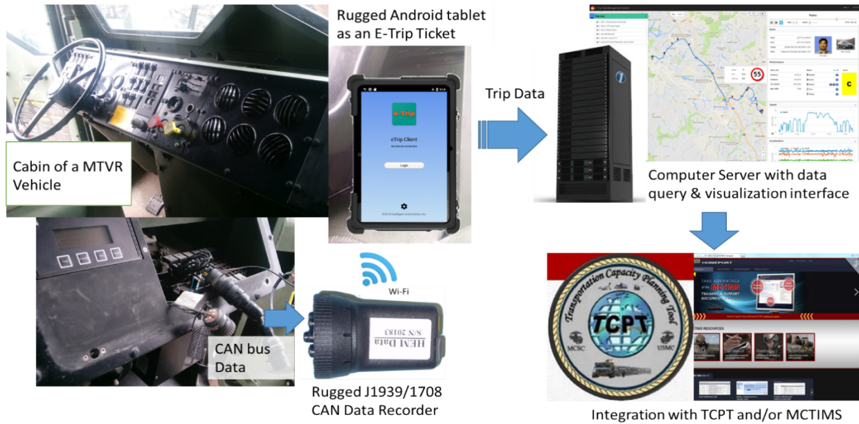
Figure 5: E-TRIP System for Vehicle Operation Performance Assessment and Vehicle Condition Monitoring
