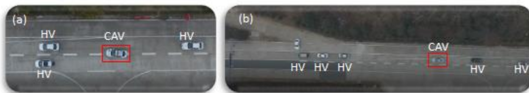
Figure 4 – Screenshots of L3 AV experiments in mixed traffic with human-driven vehicles: (a) lane changing, and (b) trajectory smooth at a traffic signal
