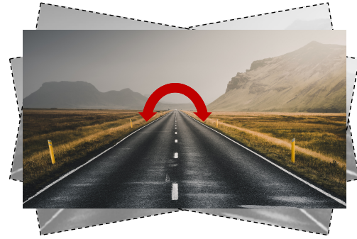
Figure 5: Rotation of Camera with respect to the roadway surface due to an uneven roadway surface.
