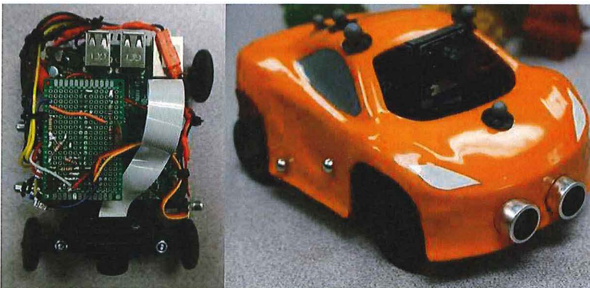
Figure 6: Vehicles used in the scaled smart city with internals (left) and outer shell (right).
