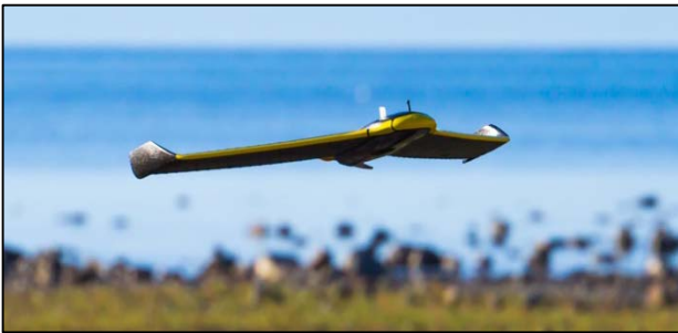
Figure 1: The senseFly eBee, a fixed-wing UAS, comes in for landing following a transportation corridor mapping project
