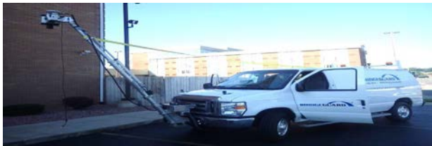
Figure 2: 3DOBS mounted alongside a thermal camera and GPS system on the BridgeGuard van
