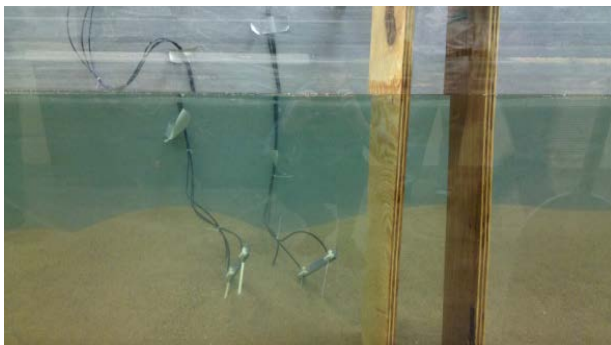
Figure 3: Laboratory scour flume study using magnetostrictive flow sensors
