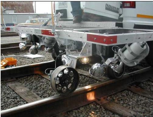
FRA is developing an automated high-resolution video joint bar inspection system that can be deployed on a hi-rail maintenance vehicle that will detect visual cracks in joint bars without having to stop the vehicle. In October 2005, a prototype system that inspects joint bars on both sides of each rail was successfully demonstrated. Testing showed that the high-resolution video system detected visual cracks that were missed by the traditional visual inspections.
