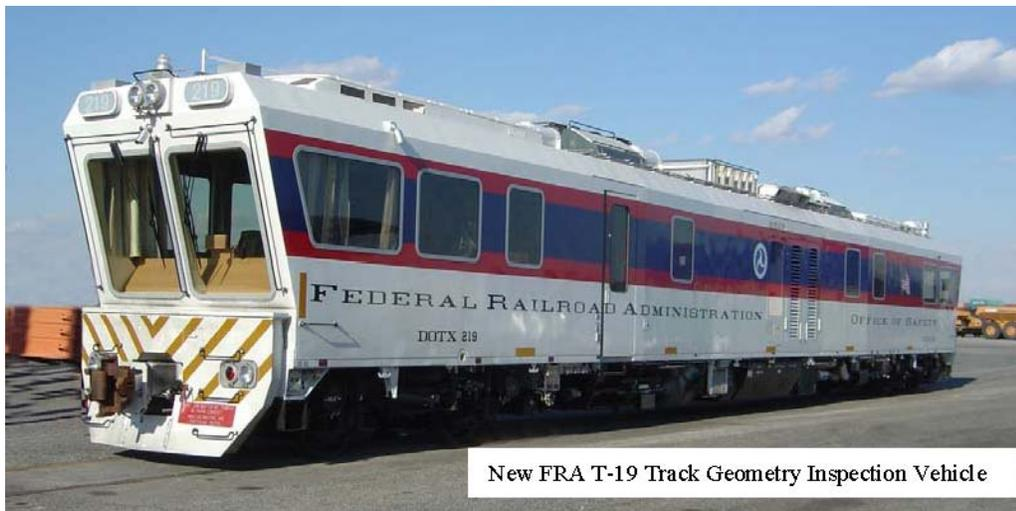
New FRA T-19 Track Geometry Inspection Vehicle
