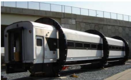
In May 2006, FRA unveiled the Passenger Rail Vehicle Emergency Evacuation Simulator, or "Rollover Rig," which can rotate a full-sized commuter rail car up to 180 degrees to simulate passenger train derailment scenarios. It provides researchers the ability to test new passenger rail evacuation strategies and safety components such as emergency lighting, doors, and windows and gives
