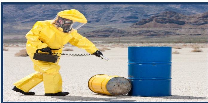
A hazardous materials worker checks for radioactivity using a Geiger counter.
