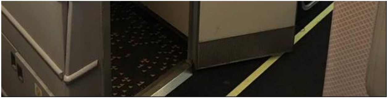
Figure 4 Photo of door sill showing 45 degree bevel. Recommended bevel should be much lower. Panel doors permit a wider open door clearance than bi-fold doors.
