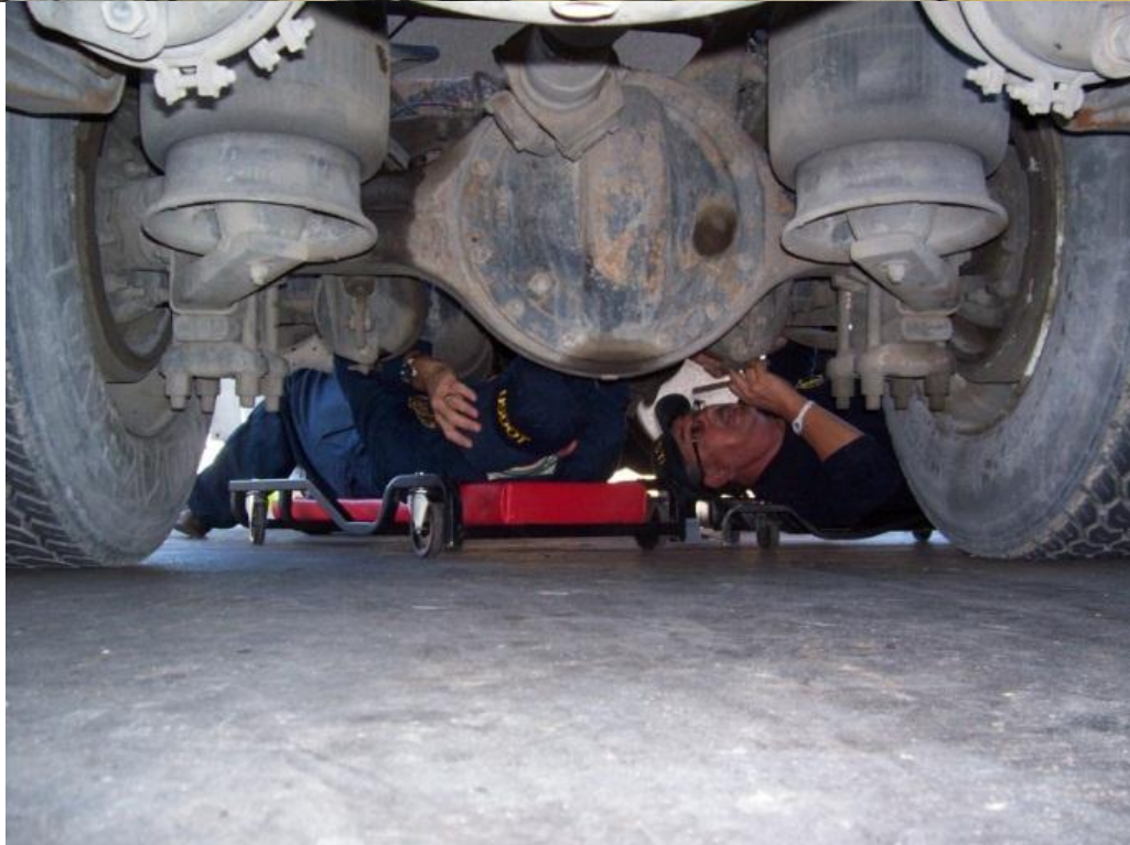
Above: The inspectors must roll under the hot truck on the hot asphalt to inspect the brakes and other functions to ensure compliance with safety regulations.
