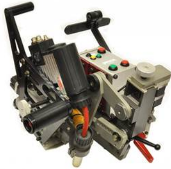
Figure 2 Courtesy of CRC-Evans - pulsed gas metal arc welding
