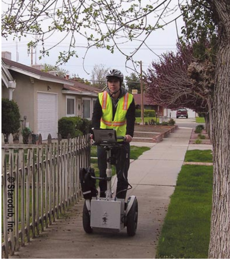
Figure 4 Sally Swanson Architects, Inc., used the Ultra-Light Inertial Profiler-ADA (ULIP-ADA™) to conduct an Americans with Disabilities Act (ADA) evaluation of sidewalk running grade, cross slope, and change in level for the City of Clovis, California.
