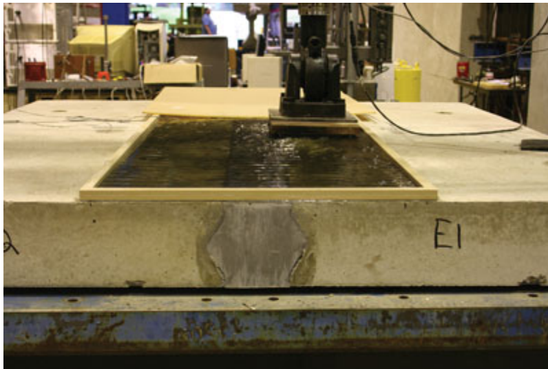
Figure 6 Ultra-high performance concrete connections are tested at FHWA's Turner-Fairbank Highway Research Center. These connections can link prefabricated bridge girders to precast concrete bridge decks.
