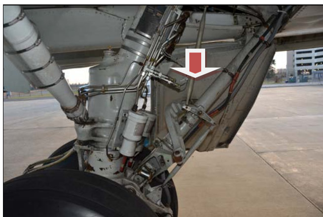
Figure 8 Image showing pressure transducers
