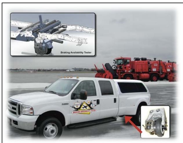
Figure 7 Braking Availability Tester
