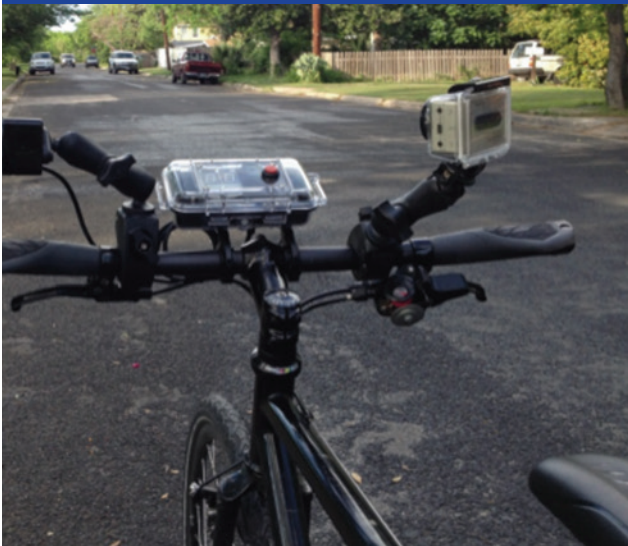
Chattanooga's BSMART/C3FT device records distances between bicycles and passing motorists for programs related to the 3-foot passing law and the Chattanooga Safe Biking Initiative.
