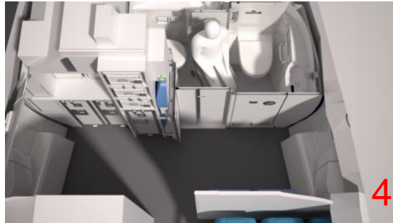
Passenger can transfer in privacy. Assisting person can enter and leave through outboard lavatory door
