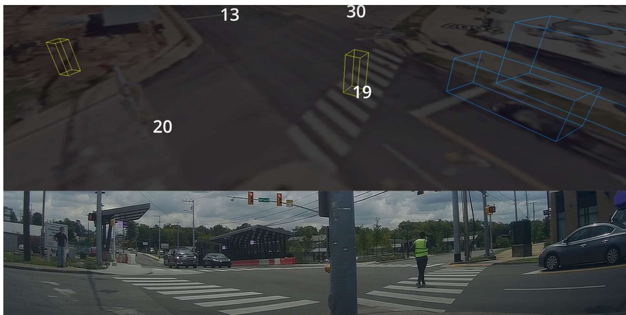
Figure 40. Single frame from the pedestrian validation study. Top. Live view of the lidar detections, with vehicles in blue and pedestrians in yellow. Numbers correspond to cumulative counts observed. Bottom. Temporary video camera used to manually annotate the pedestrian crossings for comparison to the lidar detections.
