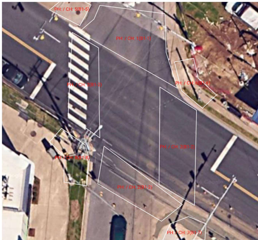
Figure 50 Pedestrian detection zones are configured in lidar software and linked to channels on a digital input/output device that can control or trigger equipment such as signal controllers or lighting.
