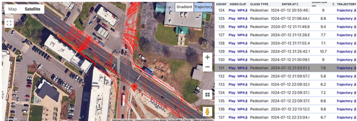
Figure 64 Out of crosswalk event log at 26 th and Clarksville Pike. Individual inspection of each trajectory and playback of conditions during the event are possible. Frequent crossings of Clarksville Pike west of the intersection and 26th Ave north of the intersection are due to nearby residents visiting convenience stores.
