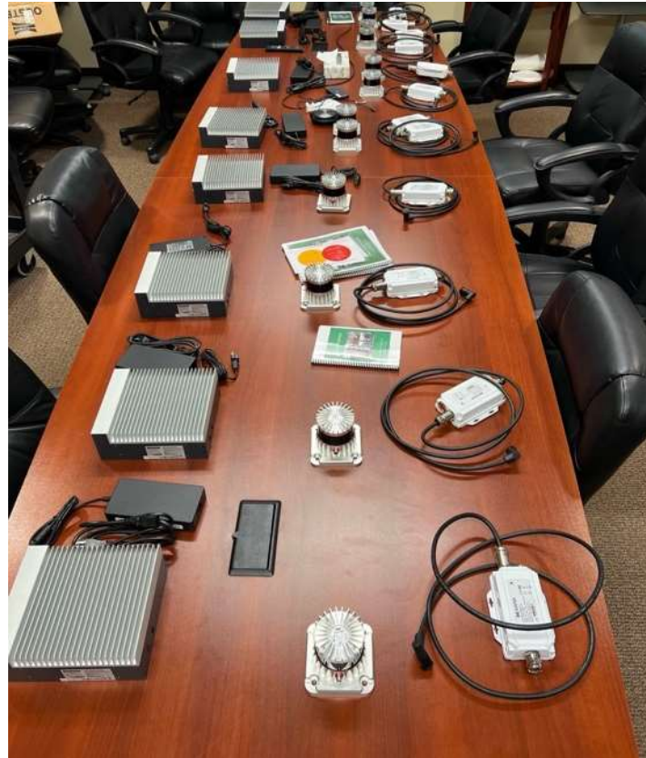
Figure 71 Stage I equipment includes an edge computer (left) a lidar sensor center, and a power supply (right). Photo taken in Stansell Electric Company Conference Room prior to deployment.
