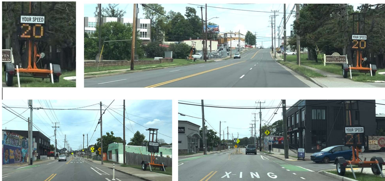
Figure 38. Midblock speeding intervention. A set of four speed trailers were placed on Clarksville Ave and Buchanan Ave. Top left: zoom in of one of the speed trailers, also shown in Top Right on Clarksville Ave. Bottom left and Bottom right show two speed trailers located on Buchanan Ave near a mid-block crossing.
