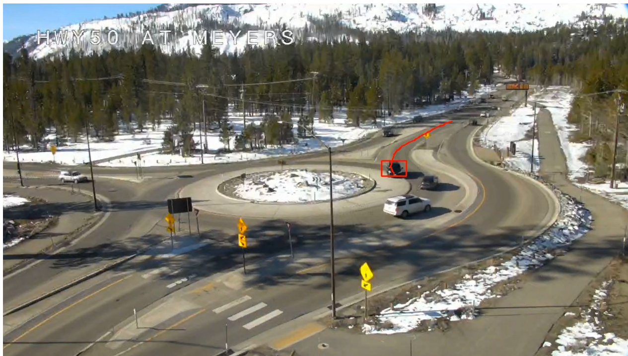
AI Sensor detection of wrong way driving
