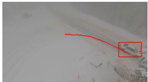
AI Sensor detecting wrong way driving in snow and low visibility conditions
