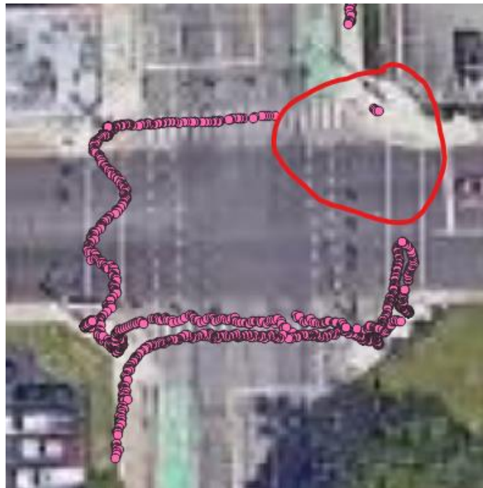
Figure 14: VRU Detection data plot that shows a blind spot in the northeast corner of the intersection due to a smudge on the camera lens.
