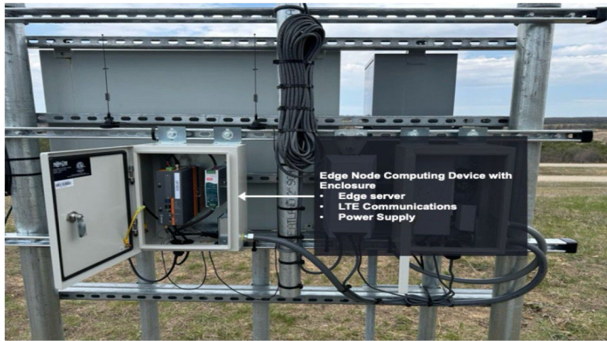
Ground Radar Tower Base Displaying the Power Supply and Server Location
