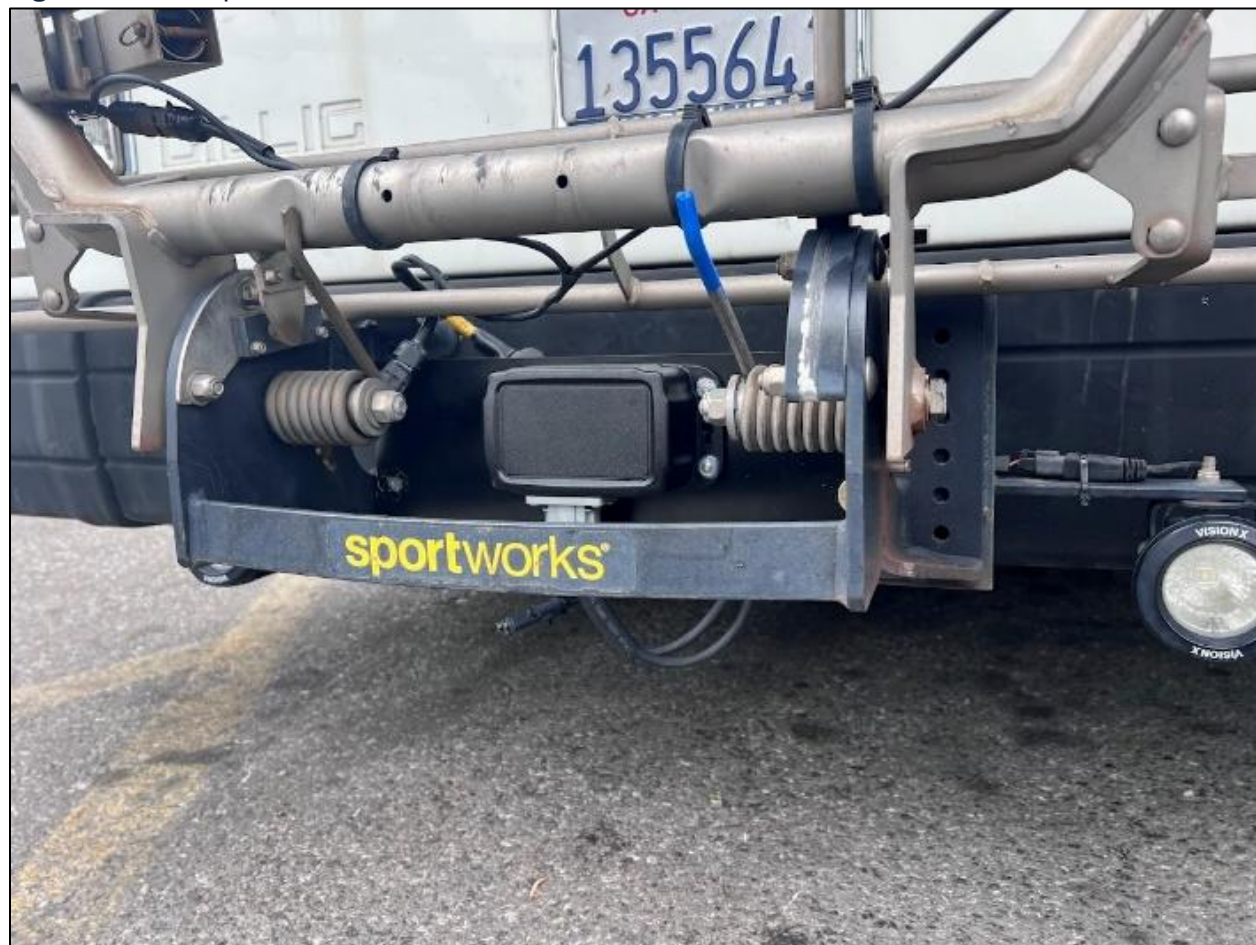
Figure 3-10. Preproduction Velolink Unit Installed on VTA Bus 4403
