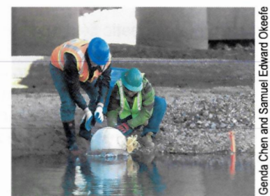
Figure 1: Two gravity-controlled N42 magnets in stack and deployment of one 135-pound smart rock in Roubidoux Creek, Missouri.
