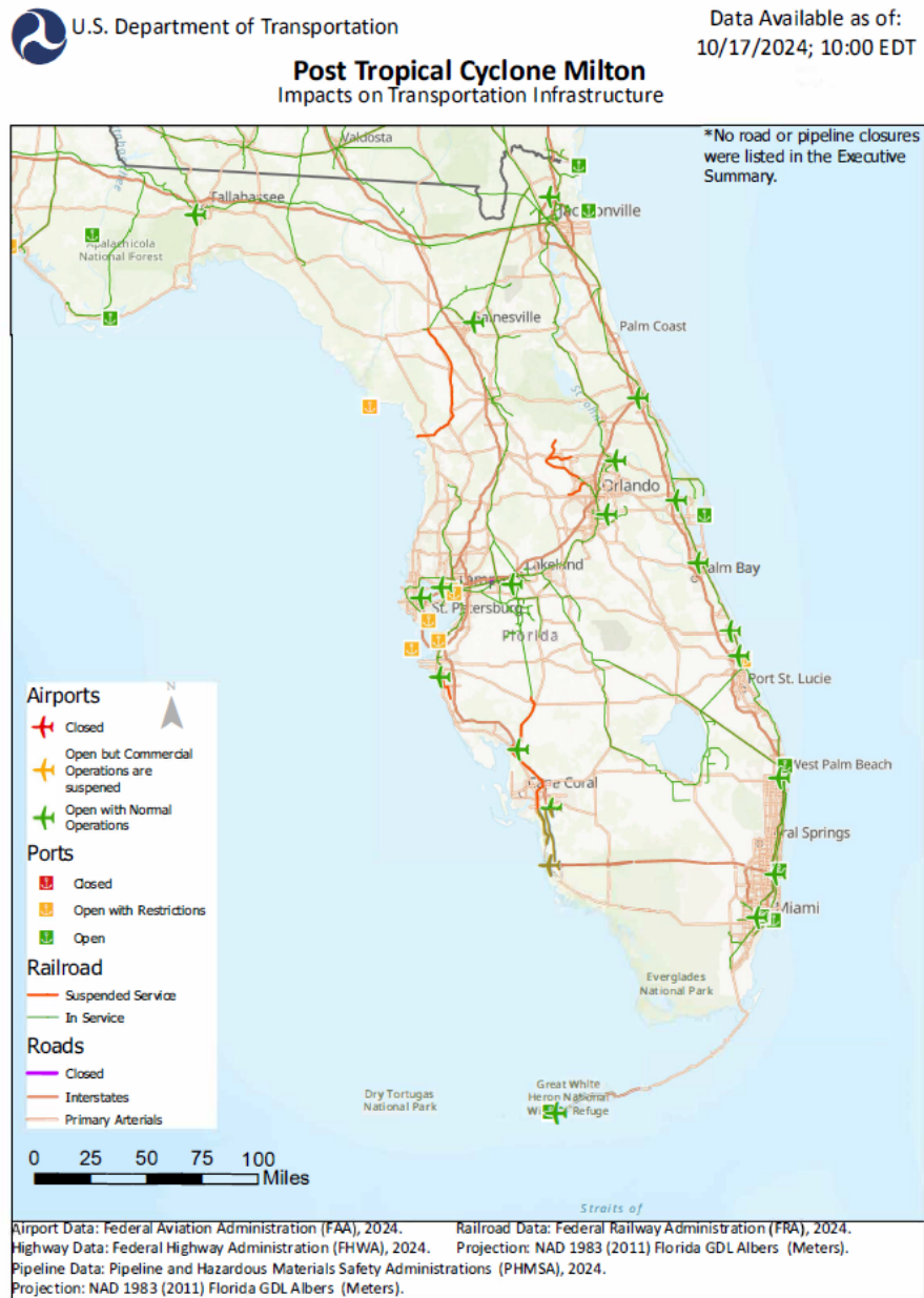
Figure 2. GIS for disaster response. This map portrays the status of transportation infrastructure during the aftermath of Hurricane Milton.
