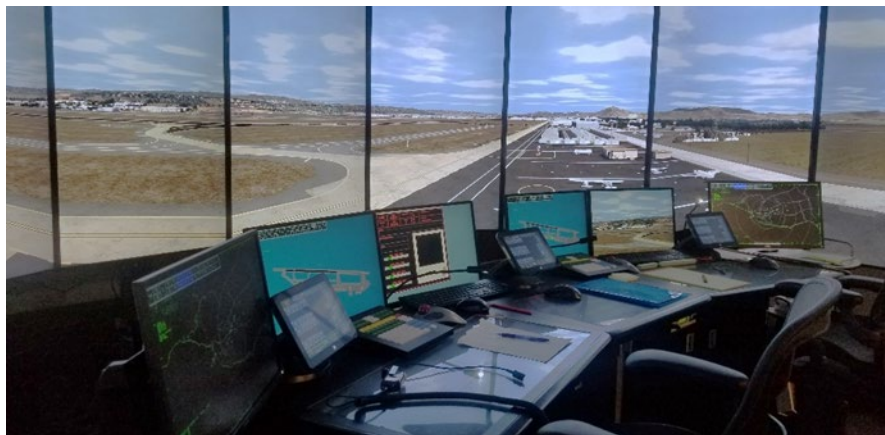
Figure 1: This is a Large Permanent TSS located in the Western Pacific Regional Office. The Visual Database shown in the simulation is of Camarillo Airport in Camarillo, California
