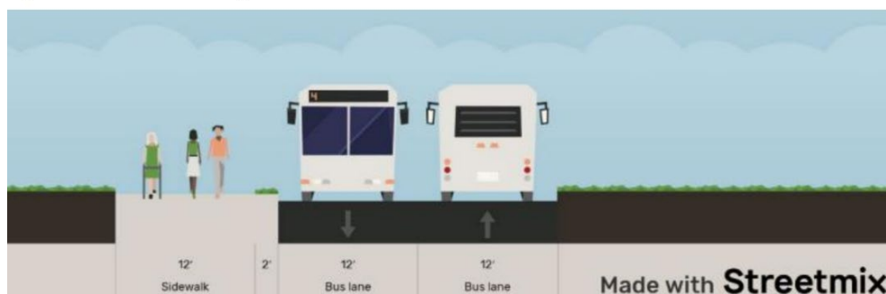
Figure 3. RFTA Rio Grande Railroad Corridor typical section #2: 23rd Street to 20th Street
