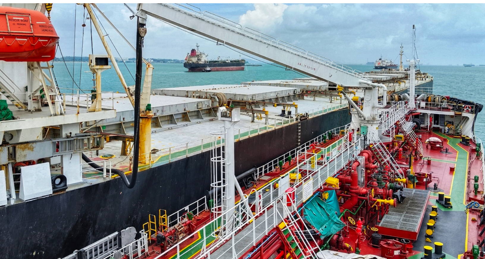
Bulk carrier (left), a type of OGV, taking on fuel from a bunkering barge (right), which is a type of harbor craft.
