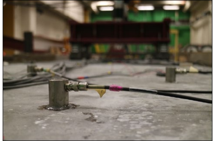
Figure 34. An acoustic emissions sensor attached to the overlay surface. Source: Tran-SET project final report
