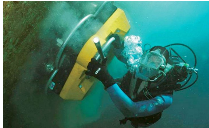
Figure 25. A diver cleaning the side of a ship. Source: Maritime Environmental Resource Center
