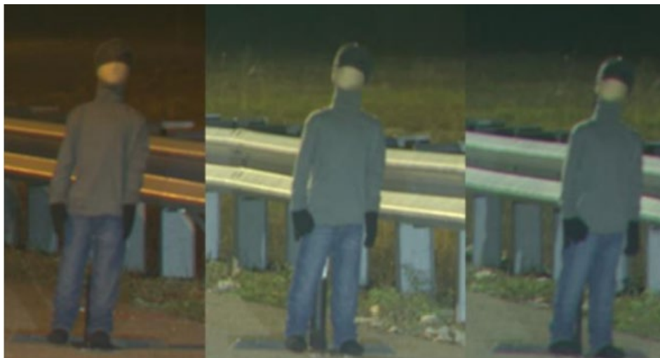
Figure 13. View of a child-sized mannequin using different light sources. Source: FHWA
