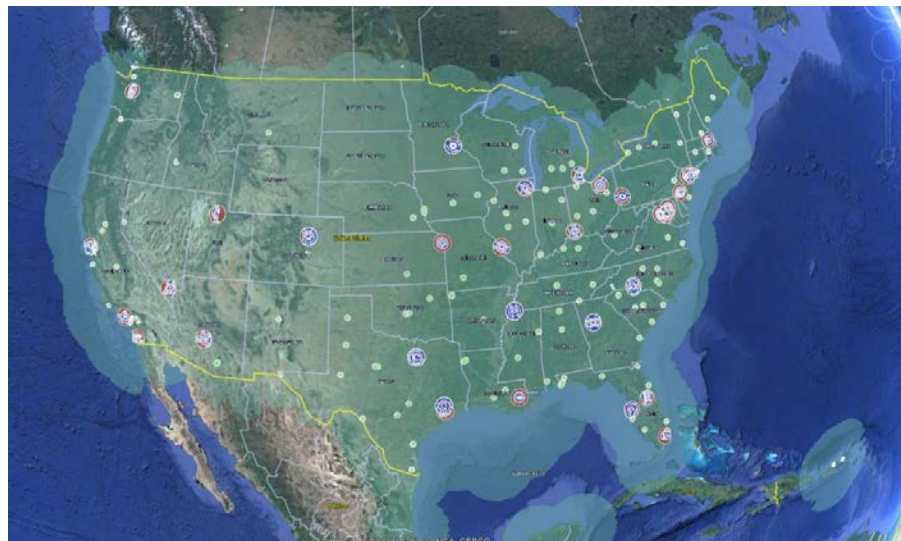
Figure 5. ADS-B coverage above approximately 10,000 ft (3,048 m).
