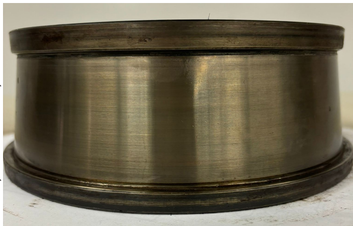
Figure 2: The inner ring (cone) raceway of bearing L7, showing no signs of damage.
