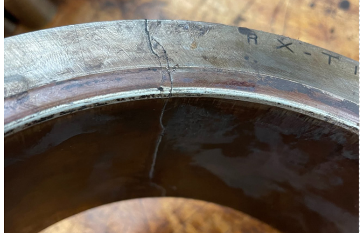
Figure 4: Fractured cone in bearing R7. This fracture could cause the cone to lose its grip on the axle, leading to indexing and catastrophic failure.
