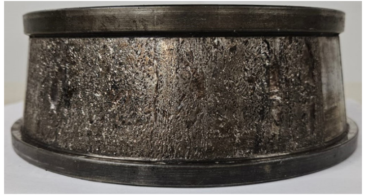
Figure 3: The inner ring (cone) raceway of bearing R7, showing severe damage over a large area.
