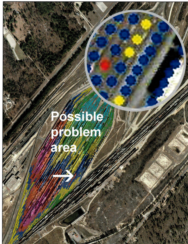
This photo shows the data collected and color coded with each color representing about one foot change in ground elevation. The data shown are available almost in real time, giving yard engineers nearly immediate feedback on where slope problems exist. Nonuniform bands of color, such as the interrupted blue band (see inset), point out problem spots.
