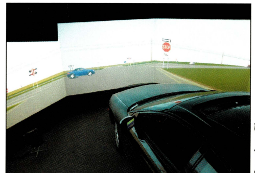
The HumanFIRST Program's immersive driving simulator enabled researchers to test a variety of infrastructure-based driver interface concepts.
