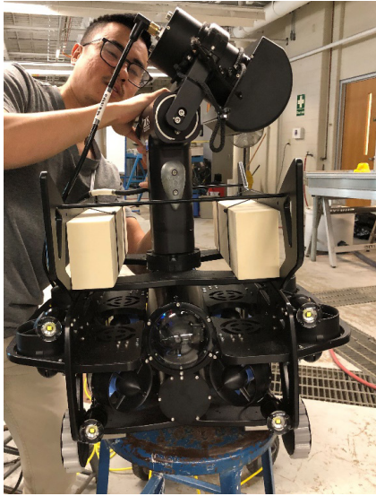
Figure 4. A hybrid swimming and roving vehicle for bridge foundation scour detection and quantification.
