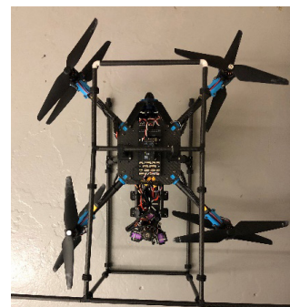
Figure 3. A hybrid flying and stationing vehicle for maintenance tasks and nondestructive tests.
