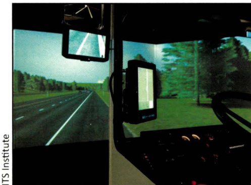
To train drivers in the proper use of the DAS, the research team constructed an immersive driving simulator that creates an accurate reproduction of a DAS-equipped bus cab.
