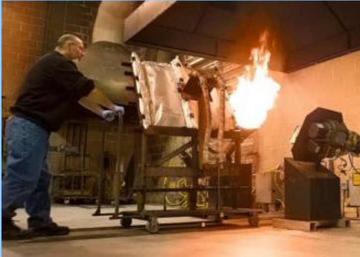
An FAA fire safety technician exposes aircraft materials to an open flame.
