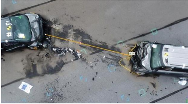
Figure 7. Using measurements from photos captured by unmanned aerial systems accelerates crash investigations. (Source: North Carolina Department of Transportation)
