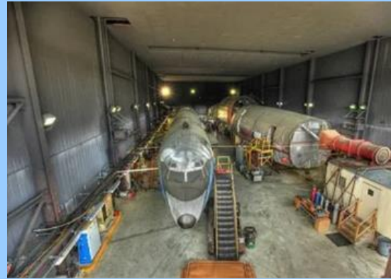
The FAA uses actual aircraft fuselages and cargo compartments to test and evaluate causes of aviation fires and the latest means of suppression and prevention.
