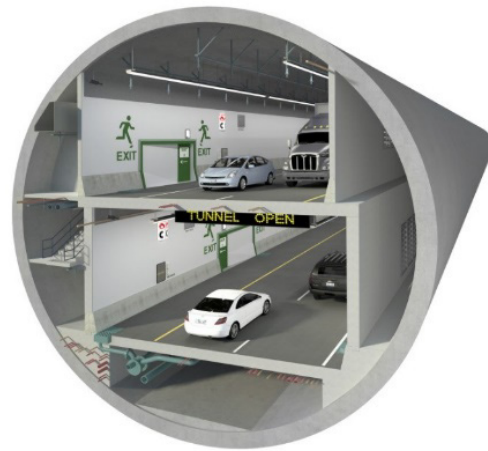
Figure 26: Design for the stacked four-lane SR-99 tunnel 322
