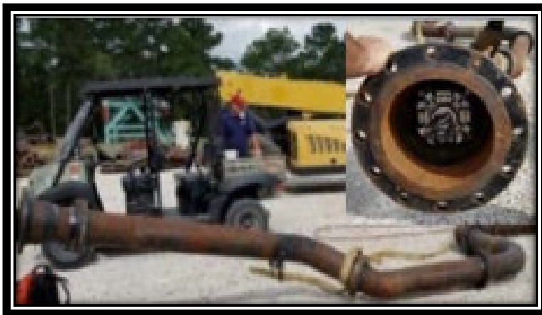
Pull testing performed by Q-Inline at testing facilities in Texas. Picture courtesy: Operations Technology Development
