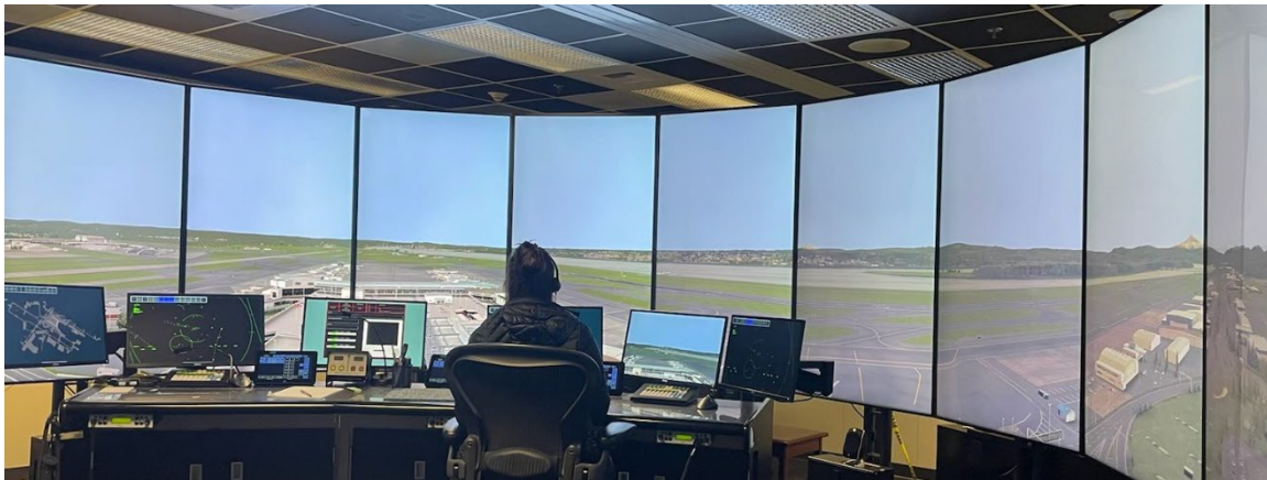
Figure 1: This is a Large Permanent TSS located in the Western Pacific Regional Office. The Visual Database shown in the simulation is of Camarillo Airport in Camarillo, California
