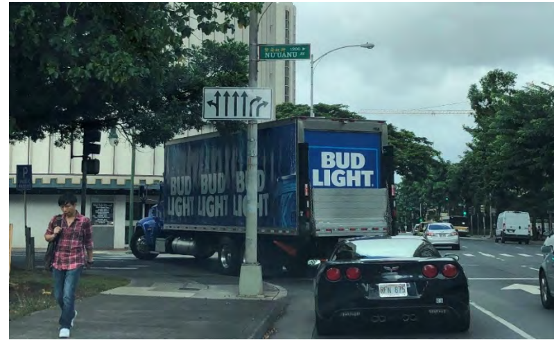
Figure 7-2. Truck Navigating a Small Radius Curb Return in Downtown Honolulu
