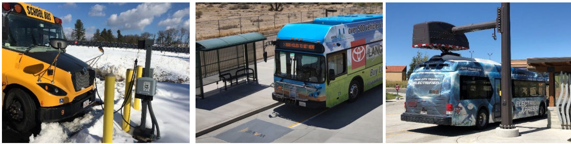
Figure 2-2: Plug-in charging (left) charges at a low power (40–125 kW) (Source: NREL/DOE, Brian Foulds/Concord-Carlisle Regional School District). Wireless inductive charging (middle) uses floor-mounted charging pads and charges at a lower power (50–250 kW), (Source: Society of Automotive Engineers ). Overhead conductive charging (right) charges at a higher power level (165–600 kW). (Source: NREL/DOE, Margaret Smith/Akimeka.
