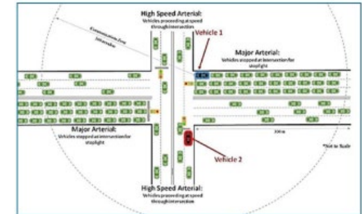
Figure 2: Test Track Scenario 2 Set-up
