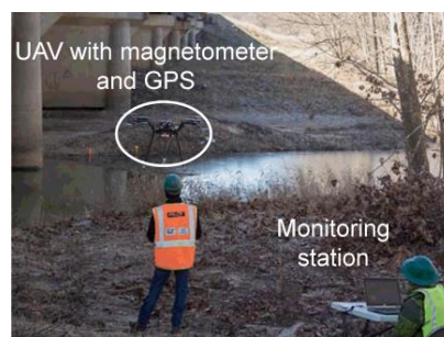
Magnetic measurement with a UAV-based sensor
