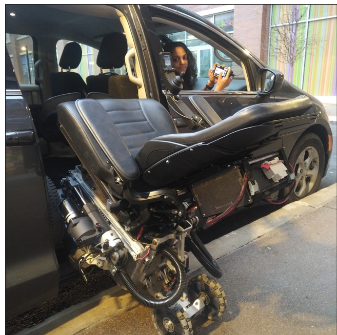
Minivan rider using remote control to operate the Mobility-Enhanced Robotic (MEBot) wheelchair. (photo credit – Jorge Candiotti)
